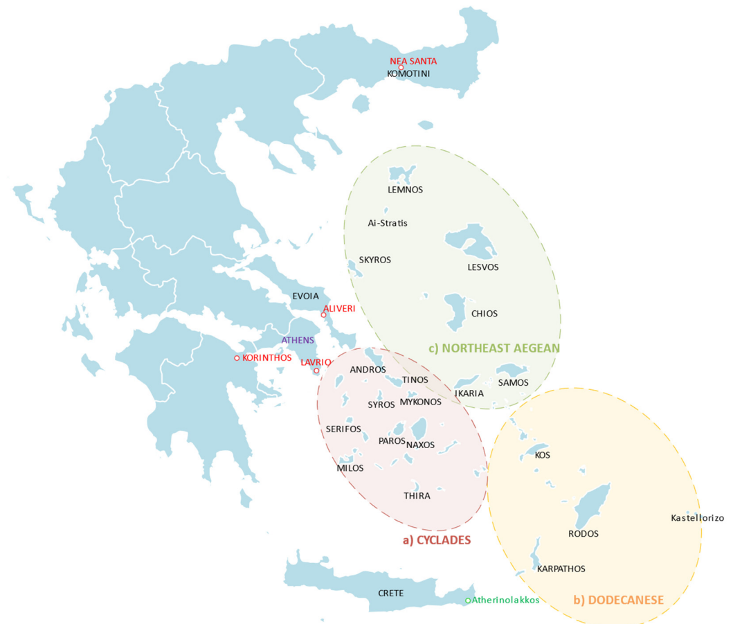
Figure 2. Map of island clusters: (a) Cycladic, (b) Dodecanese, and (c) Northeast Aegean Islands. Connection points are noted: Nea Santa, Aliveri, Lavrio, and Korinthos Extreme High Voltage Centers (EHVC) on the mainland as well as Atherinolakkos SS on Crete (under interconnection).
