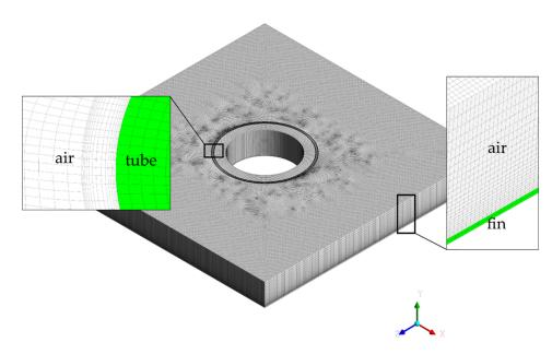
Figure 5. View of the computational mesh.
