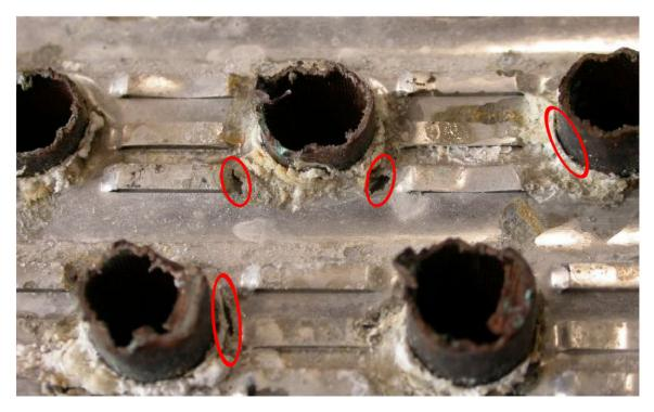
**Figure 1.** Gaps in the fin on the circumference of the tube created by a corrosion process, marked areas in the Figure (photo provided by courtesy of Blygold company [7]).
