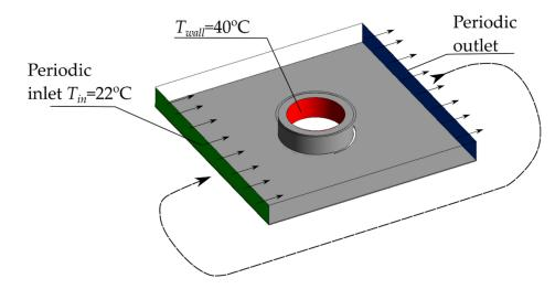
Figure 4. Boundary conditions for the computational domain.
