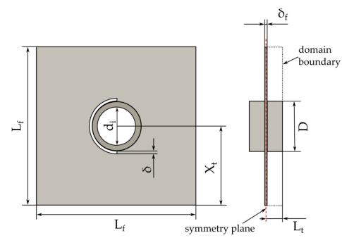
Figure 3. The geometry the simulated slice of the heat exchanger.
