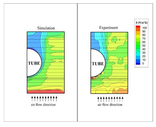
**Figure 7.** Comparison of local *h* on the surface of the fin between numerical simulation and experiment [16] for Re = 214.
