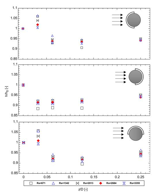
Figure 13. Heat transfer coefficient ratio in the function of dimensionless gap thickness.
