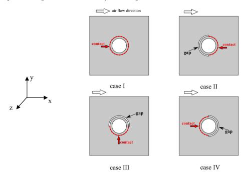
**Figure 2.** Different positions of the gap with respect to airflow: Case I—without gap; Case II—the gap in the front of the tube; Case III—the gap in the top position; Case IV—gap in the back of the tube.
