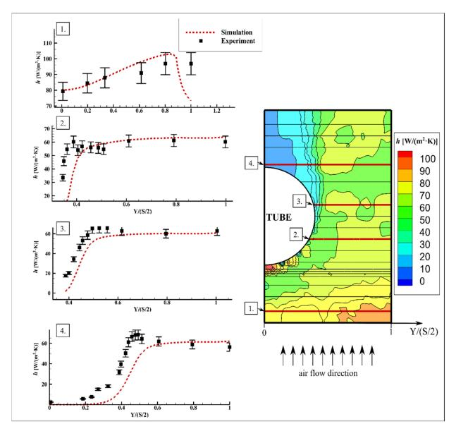
**Figure 8.** Local heat transfer coefficients from experiment versus CFD simulation at four lines transverse to the airflow at the front (line 1), back (line 4), and middle segments (lines 2, 3) of the fin for Re = 214.
