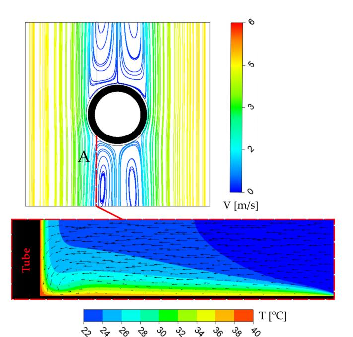
**Figure 17.** The top view of streamlines with the vector field showed on the face A upstream of the tube, at *Re* = 2013, for the ideal tube-fin contact case.
