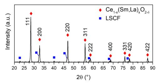
**Figure 5.** Low incidence angle (2°) X-ray diffractogram of the cathode–electrolyte interface after the selective dissolution of LSCF.
