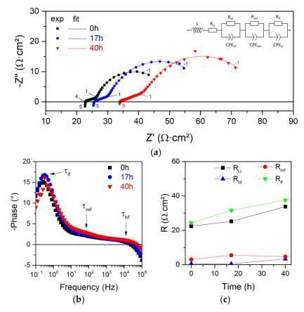
**Figure 1.** Electrochemical measurement at 550 °C of the cell sintered at 1380 °C at t = 0, 17 and 40 h (a) Nyquist plots, the numbers reported in the figure indicate the log of the frequency; (b) Bode plots; and (c) evolution of the electrolyte resistance  $R_{\Omega}$  and of the single contributions to polarization resistance  $R_{p}$  over time.
