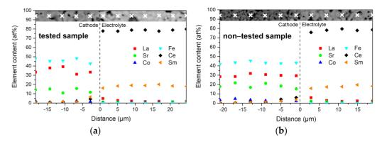
**Figure 3.** Elemental content evolution in the cathode and the electrolyte layers as a function of the distance from the interface, represented as a dashed line, for (**a**) the tested sample and (**b**) the non-tested sample. EDX point measurements were acquired at each cross on the SEM-BSE micrograph inserted at the top of the figures.
