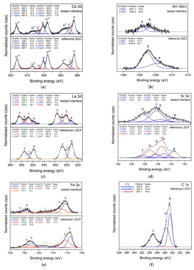
**Figure 6.** XPS windows spectra of the tested interface and the reference sample (**a**) Ce 3d core-level spectra; (**b**) Sm  $3d_{5/2}$  core-level spectra; (**c**) La 3d core-level spectra; (**d**) Sr 3d core-level spectra; (**e**) Fe 2p core-level spectra and (**f**) C 1s core-level spectra.
