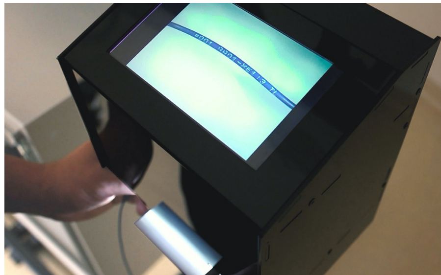
Figure 7. Wire reading with the WLR: the wire is placed by the operator on the image scene; the display on top shows the action in real time, which helps the operator to correctly place a wire.
