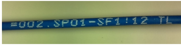
Figure 8. The picture taken by the WLR: clear, readable text; dotted font visible.
