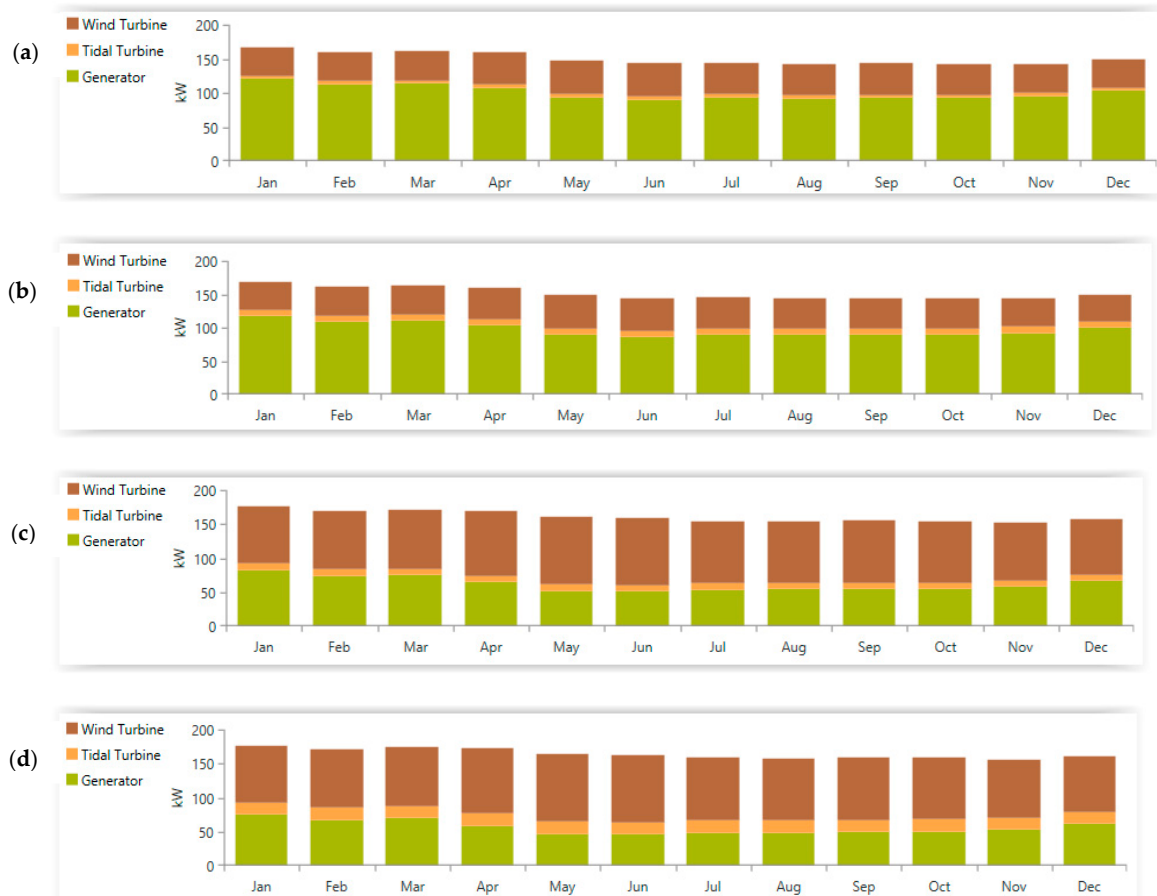
Figure 15. Monthly average output power for (a) 1W + 1T, (b) 1W + 2T, (c) 2W + 2T, (d) 2W + 4T.
