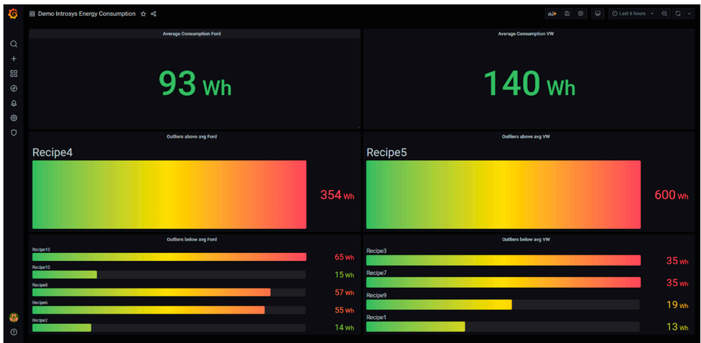
Figure 14. Energy Consumption Human Machine Interface.
