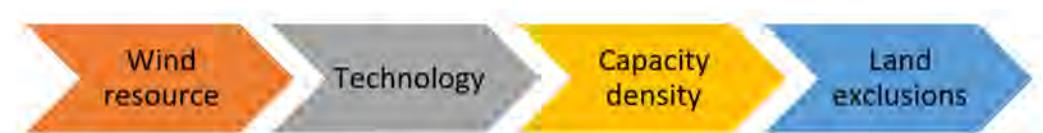
Figure 1. Major components of wind power technical potential. Turbine technology specifications determine the amount of energy that may be captured from the local wind resource. Capacity density establishes the maximum nameplate power capacity of turbines that is installable over a given area and reflects turbine spacing and siting requirements. In combination with spatial data on non-developable areas (i.e., land exclusions), these components are used to assess technical potential.
