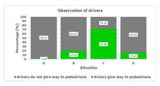
Figure 8. Results of observations of driver behaviour with regard to pedestrians in the crossing area.
