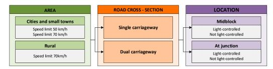
Figure 3. Diagram of test point selection.
