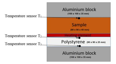
Figure 4. Temperature sensors are placed at different locations in the experimental setup.
