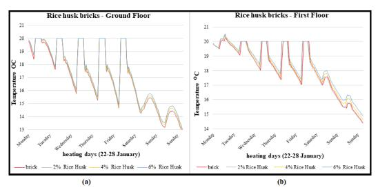
Figure 11. Ground (a) and first floor (b) heating loads using rice husk composite bricks.
