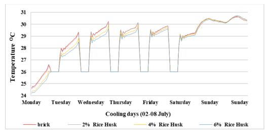
Figure 13. Ground floor cooling load using rice husk composite bricks.
