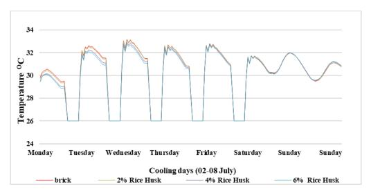
Figure 14. First-floor cooling load using rice husk composite bricks.
