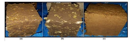
**Figure 9.** Manufactured bricks samples based on crop residue (**a**) wheat straw brick, (**b**) corn husk brick, and (**c**) rice husk brick.
