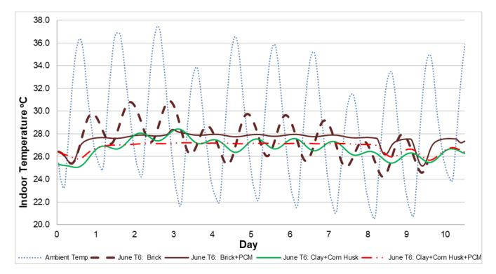
Figure 17. Simulation results depicting indoor temperature variation with outdoor ambient conditions.
