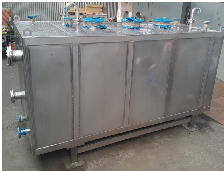
Figure 3. Thermal energy storage unit.
