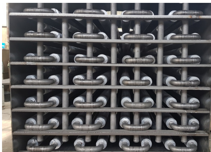
Figure 4. U-shaped charging and discharging side pipes.
