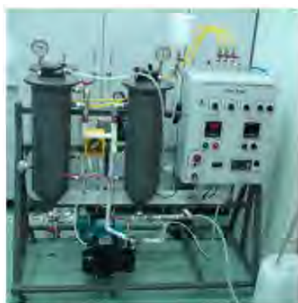
Figure 1. GW 200 reactor making vegetable oil esters to fuel diesel engines [77].
