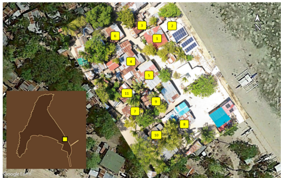
Figure 11. The household cluster of the rooftop solar microgrid showing the connected houses labelled from 1 to 11. The main image is a drone photo superimposed on Google Earth satellite imagery. The inset image shows the outline of Gilutongan Island with the yellow box indicating the solar microgrid's location.
