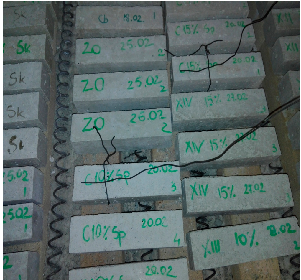
Figure 8. Mounting of thermal elements in the heating chamber before commencement of testing.
