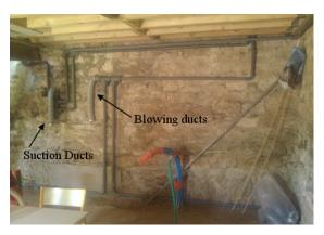
Figure 8. Instrumentation of a semi-buried wet wall.
