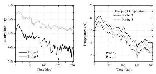
**Figure 12.** Evolution of relative humidity (**left**) and temperature (**right**) in the ventilated air space: Probe 2 was placed at the bottom of the air space while probe 3 was fixed at the top of the air space.
