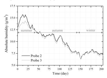
**Figure 13.** Evolution of absolute humidity in the ventilated air space: Probes 2 and 3 are fixed at the bottom and the top of the air space, respectively.
