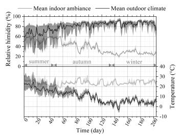
**Figure 10.** Evolution of the outdoor (black) and indoor (grey) relative humidity and temperature. Solid lines represent the daily mean measurements while shaded areas represent variations measured each day by sensors 1 and 8.
