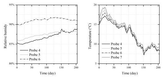
**Figure 11.** Evolution of relative humidity (**left**) and temperature (**right**) in various depths of the wet wall: Probe 4 is placed at the bottom of the wall, probe 5 at 1 m height, probe 6 at 32 cm depth and probe 7 at 1.6 m height.
