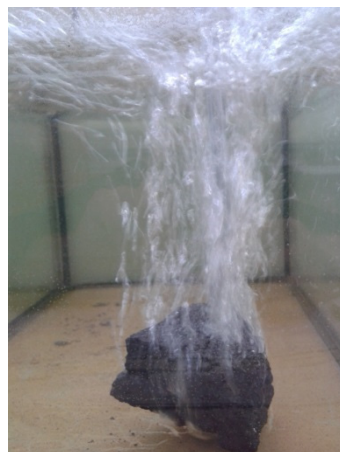
Figure 2. Flow of gas in bubbling conditions—char (I-1) [Photo by Grzegorz Wałowski].
