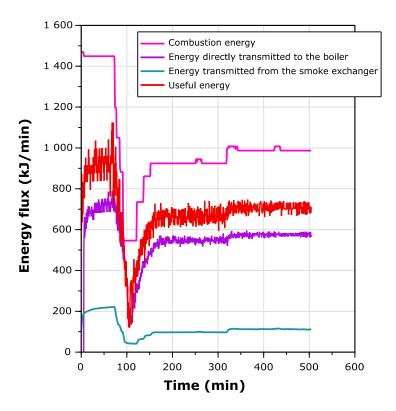
Figure 15. Time evolution of the boiler energy fluxes.
