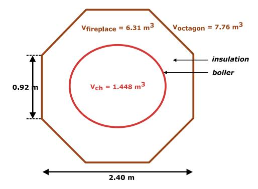
Figure 9. Sectional view of the boiler with the insulating shell.
