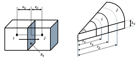
The distance between the nodes and conductivity of the materials always impact the heat transfer. In the present case, the planar element conductance is used.
