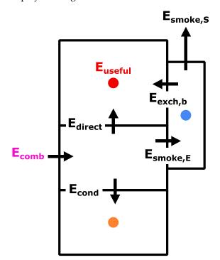
Figure 10. Final discretization of the system.
