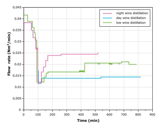
Figure 12. Gas flow rate for different types of distillation.
