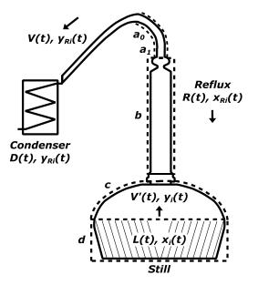
Figure 2. Scheme of the lab-scale copper still [14].
