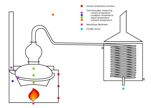
Figure 3. Instrumentation of the experimental setup.
