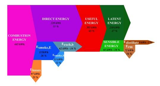
Figure 11. Sankey diagram of a wine distillation.
