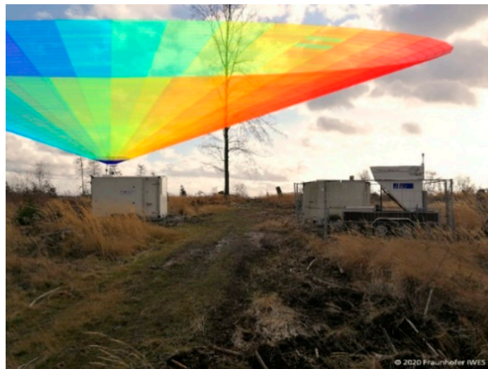
Figure 3. On-site installation of scanning lidar (left) and reference sodar (right) with illustration of scan pattern, color contours show example measurements of radial wind speed within scan. Cone angle and ranges seen here are an example used for illustration only.
