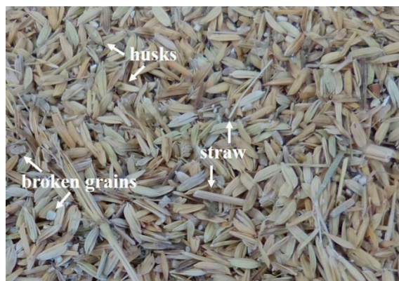
Figure 1. Photo of rice processing residue obtained in 2018 at the Rice Company 'Sur del Jíbaro' in Sancti Spíritus, Cuba. Proportion (in %weight) of the by-products: straw 1%, husk 54%, broken grains 44%.
