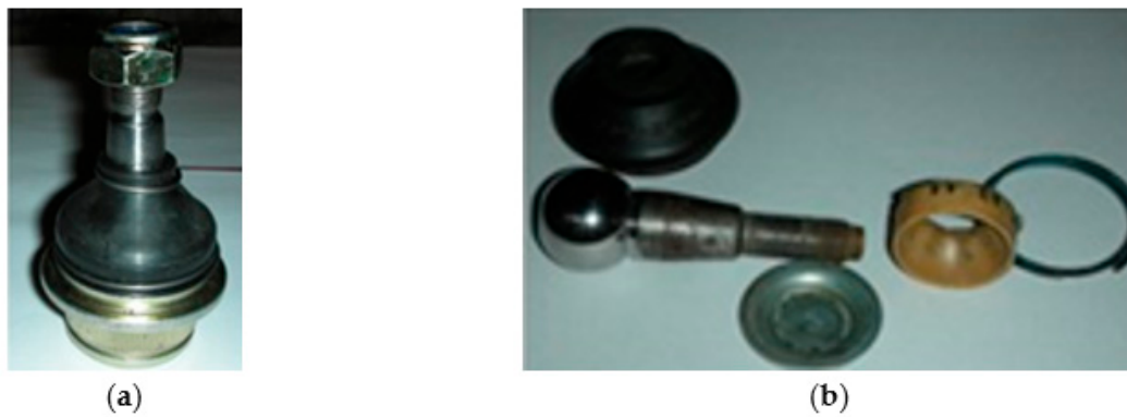
Figure 3. (a) New ball joint; (b) Disassembled used ball joint.
