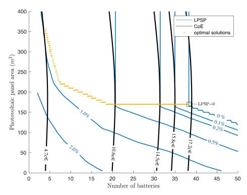
Figure 9. Photovoltaic-battery system Pareto optimal sizing.
