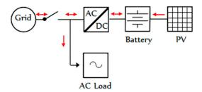
Figure 1. Simplified system power flow schematic.
