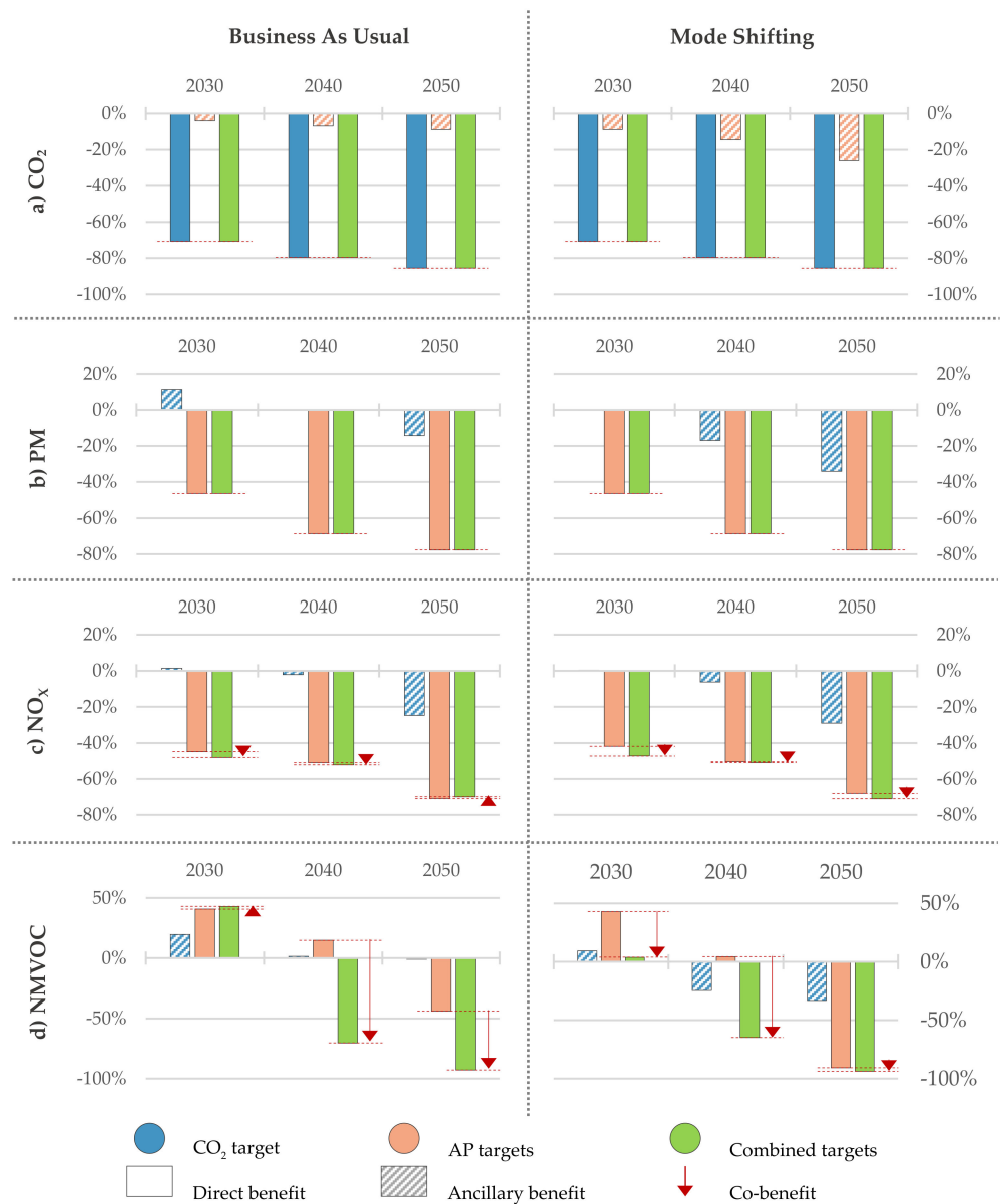
Figure 8. Additional (relative) change in emissions of (a) carbon dioxide ( \text{CO}_2 ), (b) particulate matter (PM), (c) nitrogen oxides ( \text{NO}_x ), and (d) non-methane volatile organic compounds (NMVOCs), compared with the business-as-usual reference scenario ( BAU_REF ) under different mitigation targets. Note: Solid blue bars = direct benefit for \text{CO}_2 emissions from \text{CO}_2 mitigation target; dashed blue bars = ancillary benefits for AP emissions from \text{CO}_2 mitigation target; solid red bars = direct benefits for AP emissions from AP targets; dashed red bars = ancillary benefits for \text{CO}_2 emissions from AP mitigation targets; green bars = impact of combining all mitigation targets; arrows = positive or negative co-benefits from combined mitigation targets.
