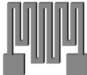
Figure 1. Schematic of meander-type Ni/Cr alloy-based microconstruction.
