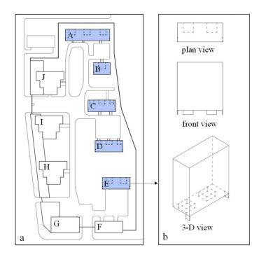
**Figure 6.** Schematic diagram of lift-up buildings: (**a**) The locations of the lift-up areas and the vertical structural elements, (**b**) schematic diagrams of the lift-up building E.
