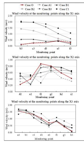
Figure 15. X1, X2, and X3 velocity measurement point wind velocities for the six cases.
