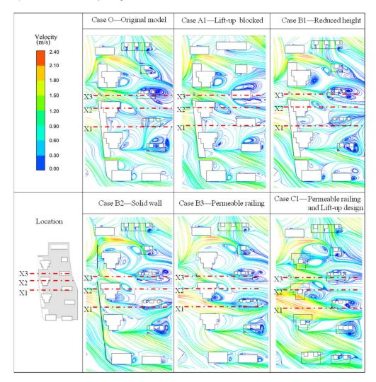
Figure 14. Streamline patterns of X1, X2, and X3 at pedestrian height for the six cases.
