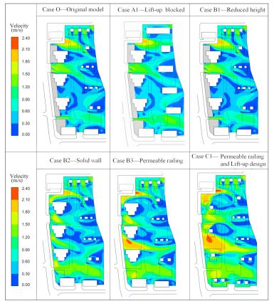
Figure 12. Wind velocity simulation results corresponding to the six cases.
