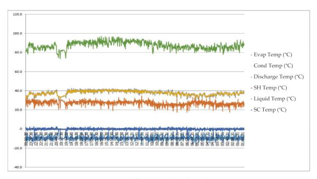
Figure 11. Temperature result for the digital-speed semi-hermetic compressor.
