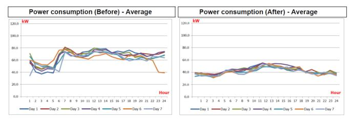
Figure 9. Average power consumption per hour before and after retrofits for store No.2 (R404A).
