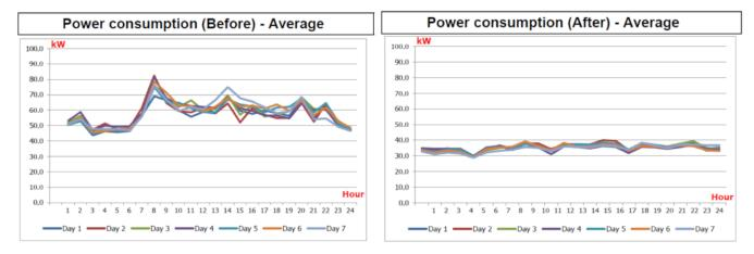
Figure 8. Average power consumption per hour before and after retrofits for store No.1 (R22).
