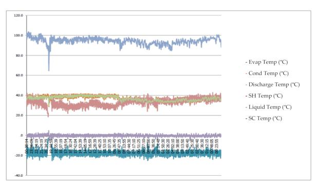
Figure 10. Temperature result for the fixed-speed semi-hermetic compressor.
