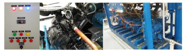
Figure 5. Digital compressor rack with digital compressor and digital controller No.1 (R404A).
