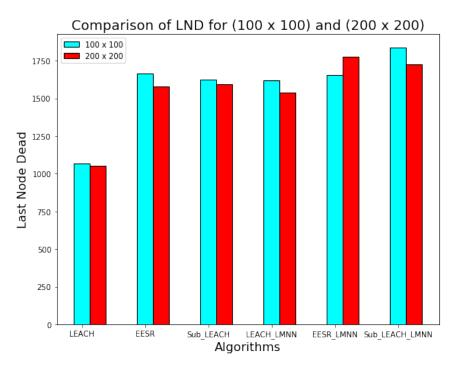
**Figure 14.** Comparison of last node dead (LND) for (100 m  $\times$  100 m) and (200 m  $\times$  200 m) for LEACH, LEACH-LMNN, EESR, EESR-LMNN, Sub-LEACH and Sub-LEACH-LMNN protocols.
