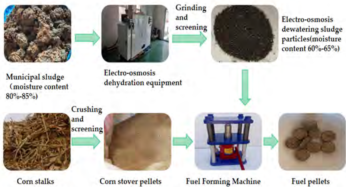
Figure 1. Compressed fuel molding process of municipal sludge mixed with corn stalks.
