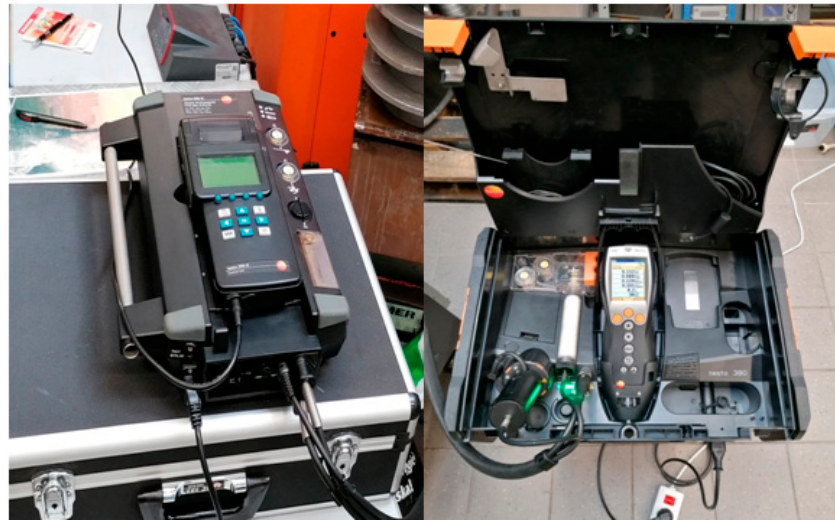
Figure 3. Exhaust gas analyzers used in tests. in left side: Testo 350s; in right side: Testo 380 and Testo 330-2 LL.
