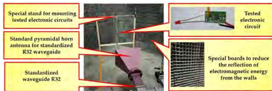
Figure 12. Special area for testing electronic devices in an electromagnetic field.
