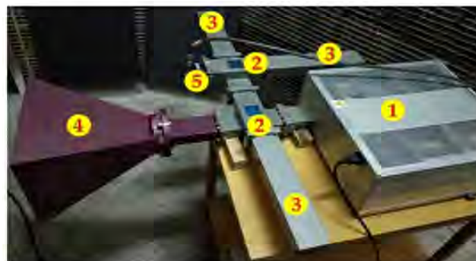
Figure 10. Assembly of a microwave power generator.
