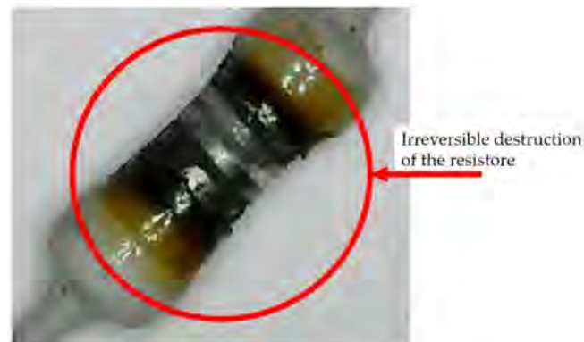
Figure 19. Irreversible destruction of the resistor.
