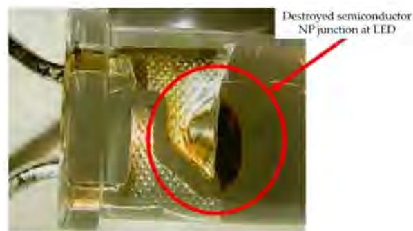
Figure 17. Detailed view of the damaged NP semiconductor structure with LED.
