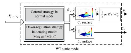
**Figure 1.** Wind turbine static model, where  $P_r$  is the power reference of the WT,  $v_e$  is the effective wind speed,  $\beta$  is the pitch angle,  $\lambda$  is the tip speed ratio,  $C_p$  is the coefficient of the power,  $\rho$  is the air density, *R* is the radius of the rotor of the turbine, and *P* is the power output.
