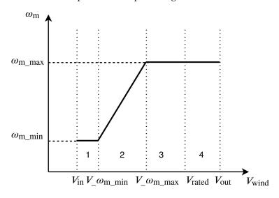
Figure 6. Speed curve based on four speed regions.
