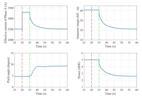
Figure 12. Waveforms of the main variables of the faulty generator.
