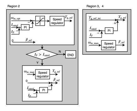
**Figure 7.** Flowchart of the ITSC FRT strategy, where  $I_F$  is the current of the faulty phase,  $I_{rated}$  is the rated current,  $T_{g\_ref\_ini}$  is the generator torque reference the initial torque controller,  $\omega_{m\_max}$  is the maximum rotor speed,  $\beta_{ref}$  is the pitch angle reference, and  $\omega_{m\_opt}$  is the optimal rotor speed according to MPPT.
