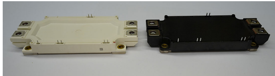
Figure 4. Selected half-bridge modules: (Left) (1700 V, 250 A) Infineon FF300R17ME4 (SI-IGBT + Si-Diode) [19]; and (Right) (1700 V, 250 A) Rohm BSM250D17P2E004 (SiC-Mosfet+SiC-SBD) [20].
