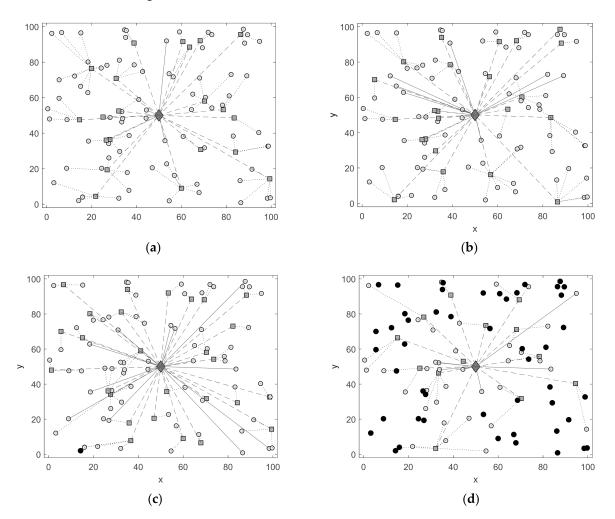
**Figure 4.** Wireless sensor network clustering evolution: (**a**) cluster configuration in round 1, (**b**) in round 5, (**c**) in round 11, and (**d**) in round 15.
