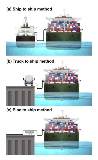
**Figure 2.** LNG Bunkering methods: (**a**) ship to ship method, (**b**) truck to ship method, and (**c**) pipe to ship method.
