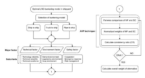
Figure 4. AHP framework for optimal LNG bunkering model in shipyard.
