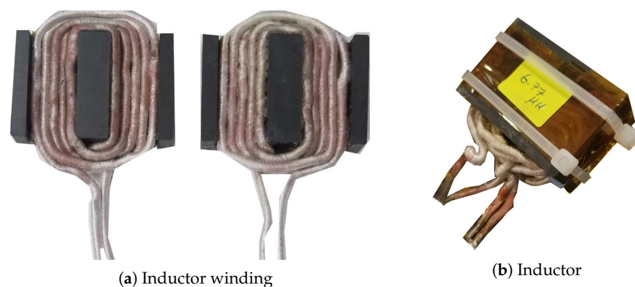
Figure 10. View of inductor (E38/8/25 core, 3F36 material, 6.8 \mu\text{H} inductance).
