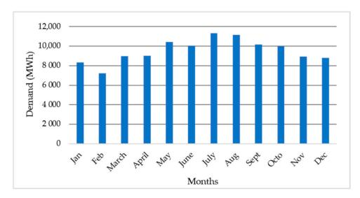
**Figure 11.** Total electricity demand on Isla de la Juventud in different month of 2019 Source: own elaboration with the model [27].
