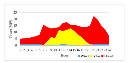
**Figure 18.** Electricity production for a day (19 April 2030) for the RENES scenario. Source: own elaboration with the model.
