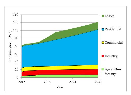
**Figure 15.** Electricity consumption of Isla de la Juventud in 2030 in the RENES scenario. Source: own elaboration with the model [27].
