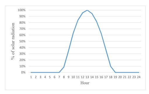
**Figure 5.** Hourly solar radiation curve for one day in Isla de la Juventud. Source: own elaboration with the model [28].
