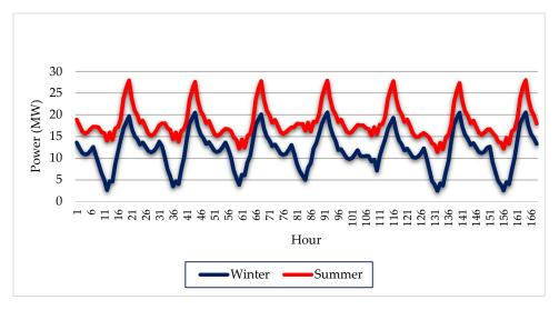
**Figure 19.** Residual load curve for a typical winter week versus summer week in 2030 for the RENES scenario. Source: own elaboration with the model.
