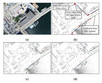
**Figure 9.** The process of matching the land area lines generated from the ENC to the edges detected in the image: (a) Source image; (b) Step 1 of iteration,  $l_1 = 115$  pixels,  $\sigma_1 = 3^{\circ}$ ; (c) Step 2 of iteration,  $l_2 = 58$  pixels,  $\sigma_2 = 1.5^{\circ}$ ; (d) Step 8 of iteration,  $l_8 = 1$  pixel,  $\sigma_8 = 0.023^{\circ}$ .
