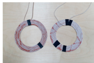
Figure 19. Fabricated actual WPT coils.
