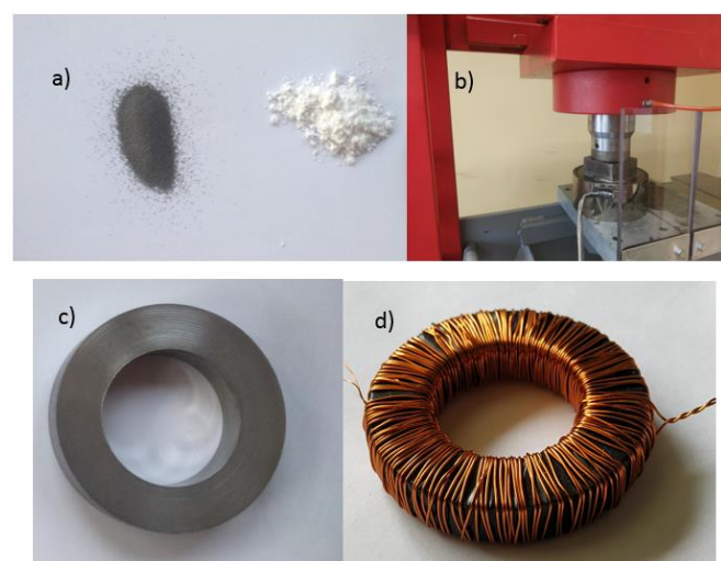
Figure 1. Illustrative steps in the production of composite core samples: (a) components, (b) forming, (c) produced core, (d) core with windings.
