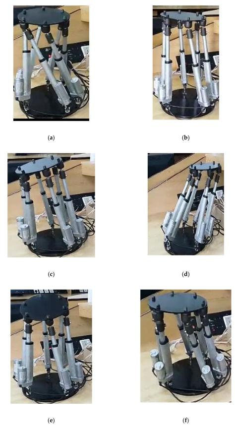
**Figure 15.** (a) Rotation in Z-Axis, (b) Translation in Z-Axis, (c) Rotation in Y-Axis, (d) Translation in Y-Axis, (e) Rotation in X-Axis, (f) Translation in X-Axis.
