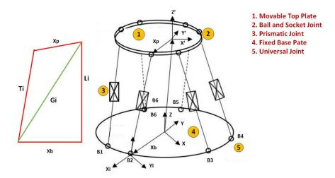
**Figure 3.** Schematic and vector representation of the proposed machining bed. (**Right**) schematic representation of kinematic chain connections and angle distribution. (**Left**) the schematic diagram for the ith leg of the mechanism.
