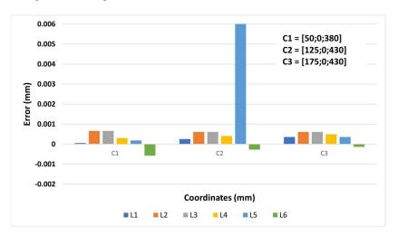
Figure 18. Error in leg lengths of six legs (L1 to L6) for three different tests positions (C1, C2 and C3).
