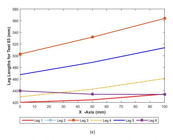
**Figure 10.** (a). Leg Length obtained for test 01 (Leg 2 and Leg 3 have same lengths); (b). Leg Length obtained for test 02 (Leg 2 and Leg 3 have same lengths); (c). Leg Length obtained for test 03 (Leg 2 and Leg 3 have same lengths).
