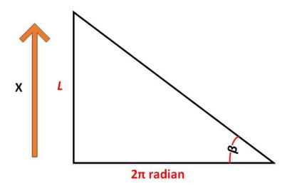
Figure 7. Relationship between angular and linear movement of linear actuator.
