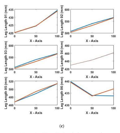
**Figure 17.** (a) Actual and desired leg lengths during test 01 for experimental validation; (b) Actual and desired leg lengths during test 02 for experimental validation; (c) Actual and desired leg lengths during test 03 for experimental validation.
