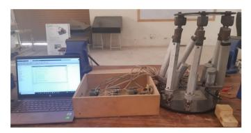
Figure 14. Fabricated model of the six DOF machining bed.
