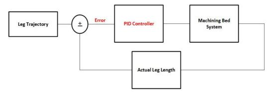
Figure 12. Block diagram of the feedback control model for the machining bed.
