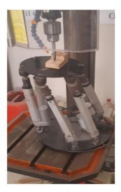
**Figure 16.** Experimental setup. (A pictorial view of the test being carried out by machining bed on a workpiece).
