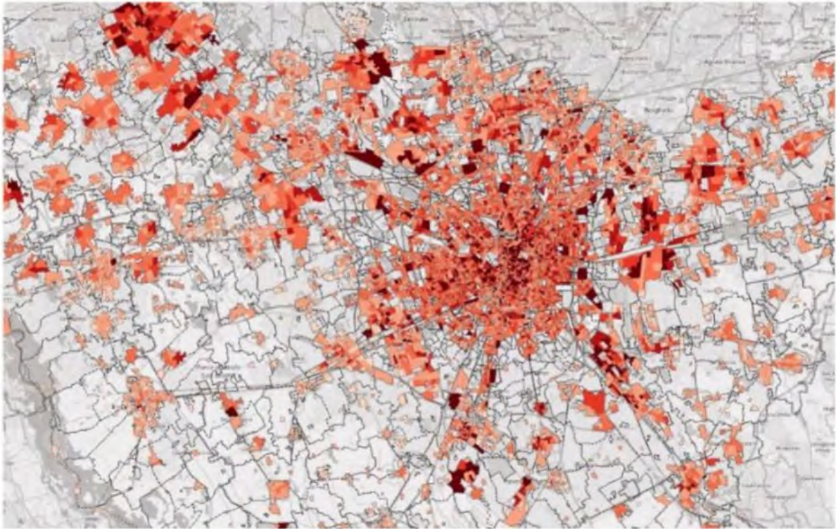
Figure 13. Map of the census areas with an associated specific distribution total cost lower or equal to 50 €/MWh. Scenario 1.
