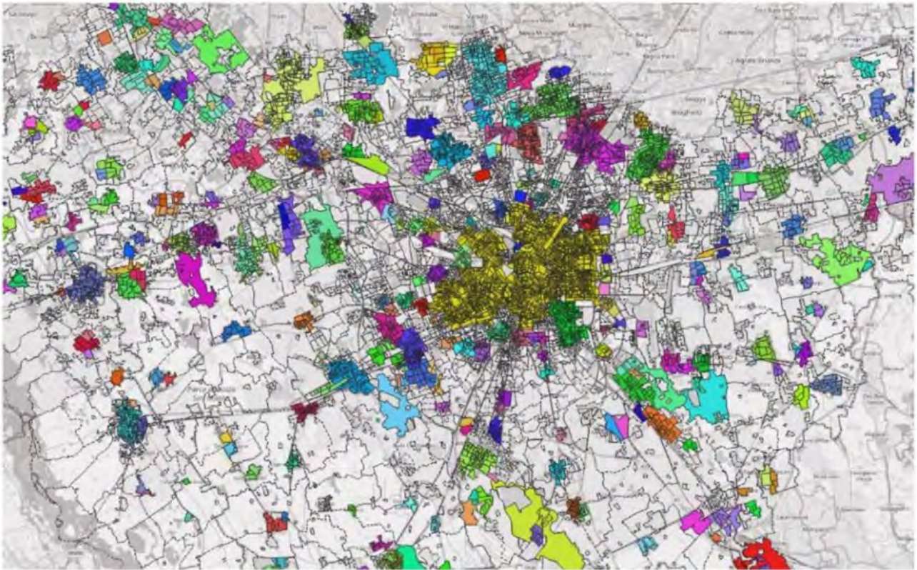
Figure 7. Map of the province of Milan, with the generated heat demand clusters distinguished by color. Scenario 1.
