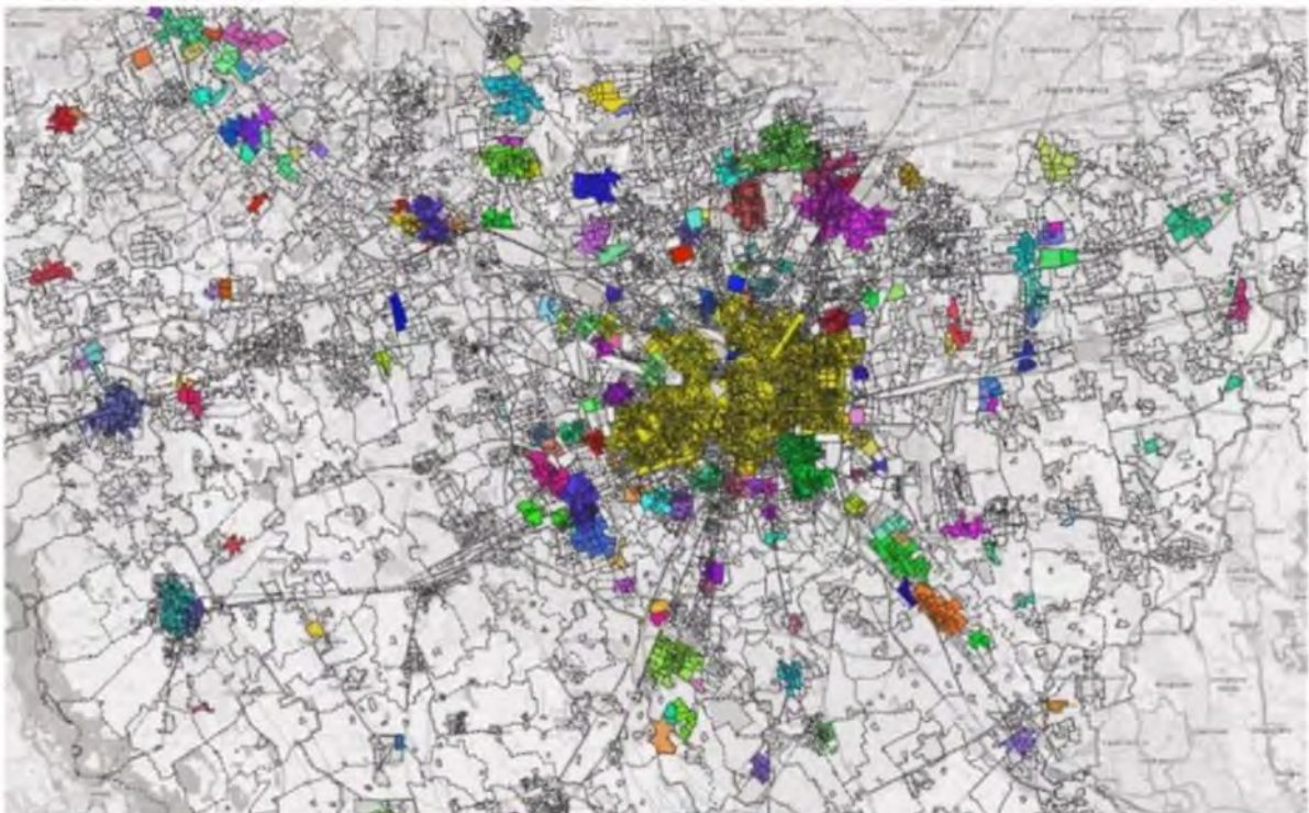
Figure 14. Map of the clusters with an associated specific distribution total cost lower or equal to 50 €/MWh. Scenario 1.
