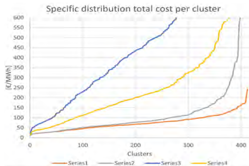
Figure 15. Average specific distribution total cost per cluster. Curves are constructed for each studied scenario by ordering the values in ascending order.
