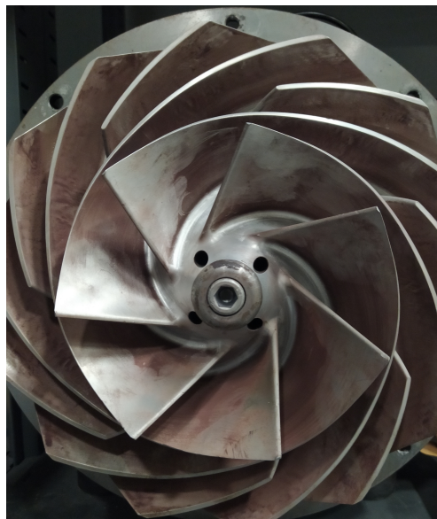
Figure 4. Manufactured SR impeller.
