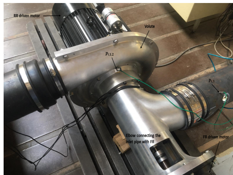
Figure 14. View of the CRCC with the position of two Kistler probes.
