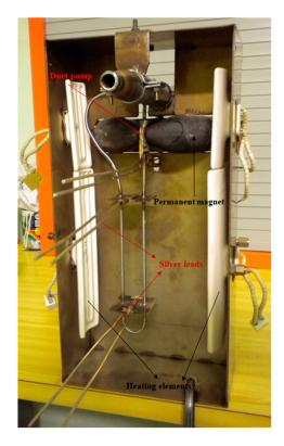
Figure 1. Picture of the current resistivity meter.
