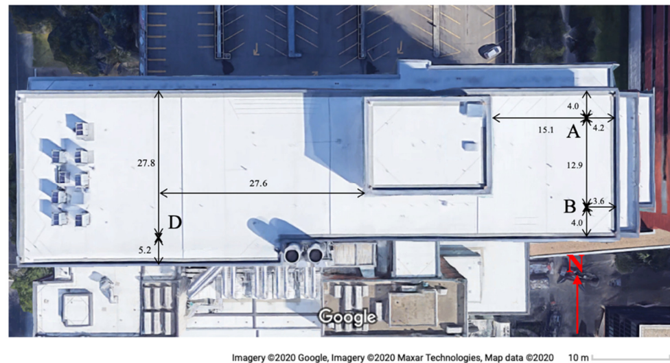
Figure 6. Locations of anemometers on the roof of the Donadeo ICE building. Note that dimensions are in m.
