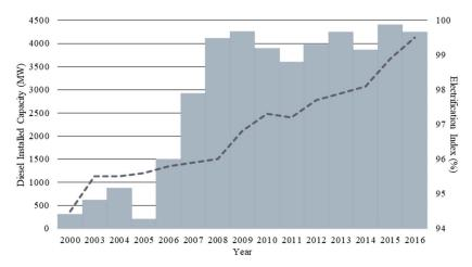
Figure 2. Growth in installed capacity of generator sets and electrification rate in Cuba.
