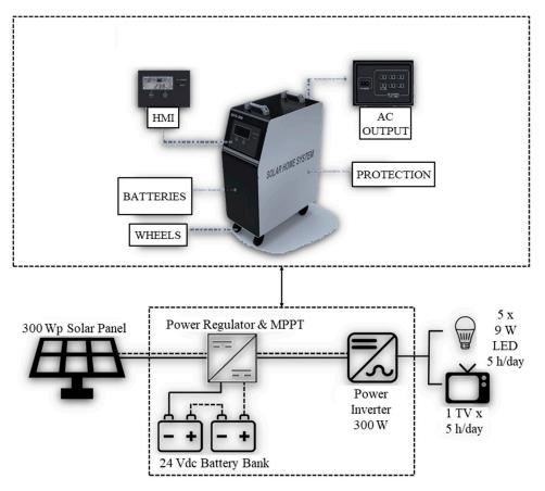
Figure 5. Electrical scheme of a modular solar system installed in Río Abajo.
