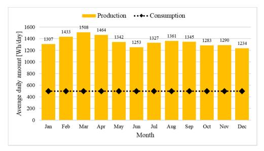
Figure 8. Typical daily performance of a PV-based system installed in Río Abajo (kWh/day).
