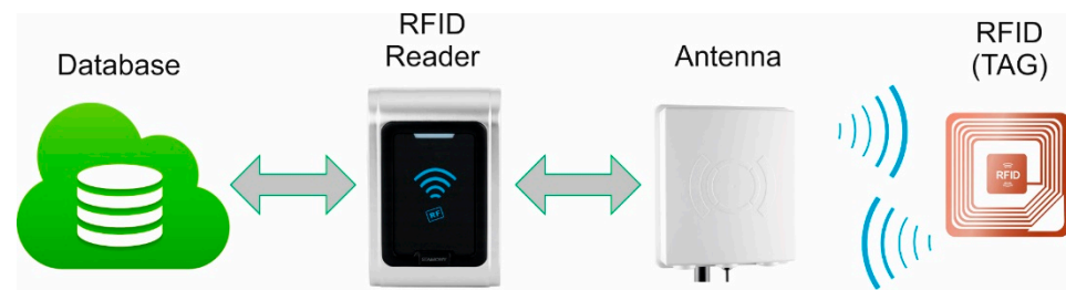
Figure 4. The structure of the system using RFID tags.
