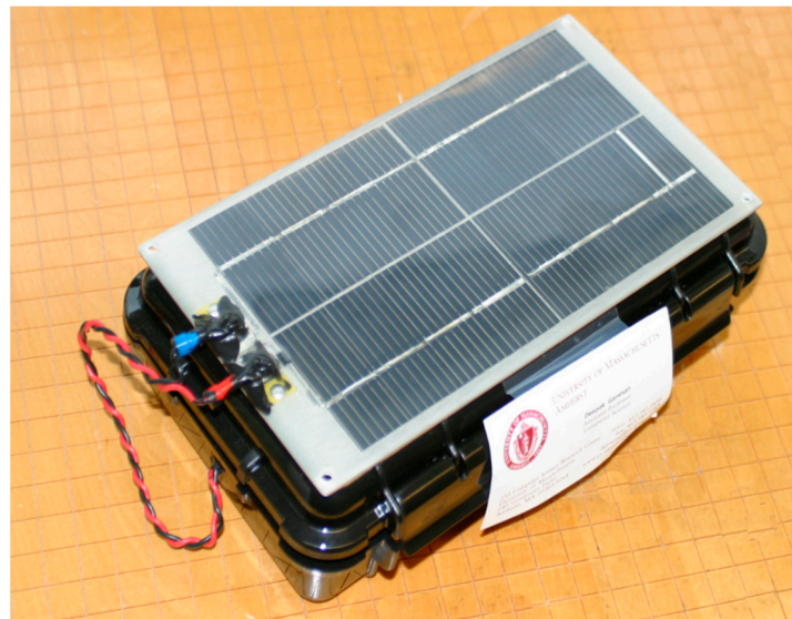
Figure 11. Measurement node using a photovoltaic panel [34].
