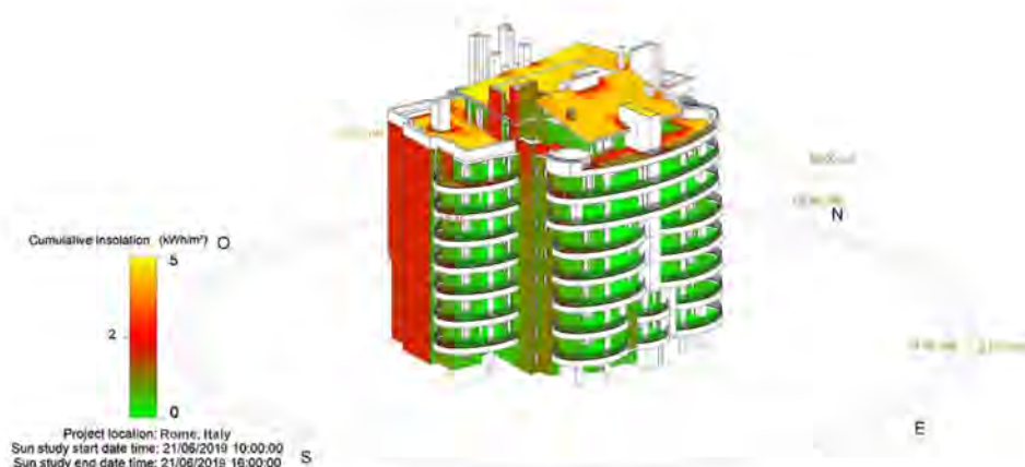
Figure 9. Solar radiation analysis.
