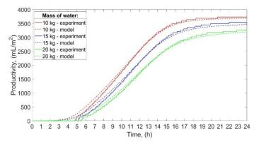
**Figure 8.** The productivity of the solar still for different masses of water and medium power of the electric heaters.
