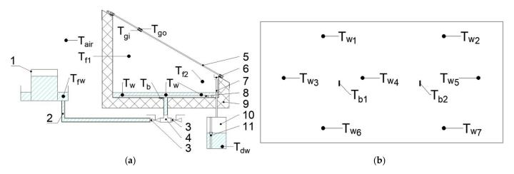
**Figure 1.** Diagram of the investigated solar still: (a) Cross-section; (b) Top view. 1—feeding water tank; 2—pipe system; 3—shut-off valve; 4—three-way valve; 5—glass cover; 6—distillate trough; 7—distillate channel; 8—electric heater; 9—thermal insulation; 10—distillate tank; 11—water level sensor; T—locations of the temperature sensors (the readers are referred to Nomenclature for details of subscripts).
