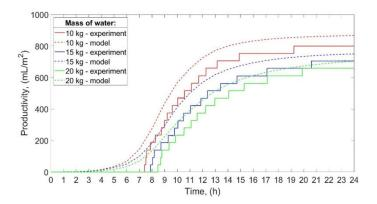
**Figure 6.** The productivity of the solar still for different masses of water and low power of the electric heaters.
