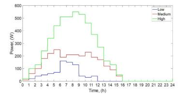
Figure 3. Power of the electric heaters in the function of time.
