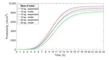
**Figure 10.** The productivity of the solar still for different masses of water and high power of the electric heaters.
