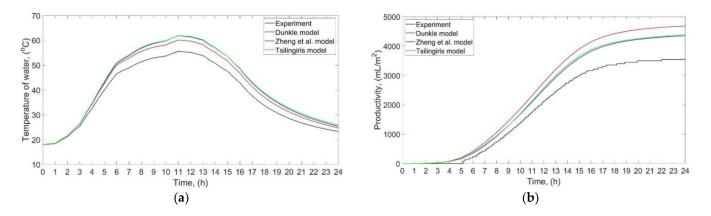
**Figure 4.** Comparison of the results of experiments and three mathematical models for 15 kg of water and medium power of the electric heaters: (a) Water temperature; (b) Productivity.
