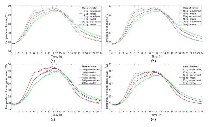
**Figure 7.** Temperatures of: (**a**) Water; (**b**) Basin; (**c**) Inner glass cover; (**d**) Outer glass cover; obtained experimentally and theoretically in the function of time for different water masses and medium power of the electric heaters.
