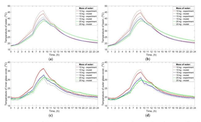
**Figure 5.** Temperatures of: (**a**) Water; (**b**) Basin; (**c**) Inner glass cover; (**d**) Outer glass cover; obtained experimentally and theoretically in the function of time for different water masses and low power of the electric heaters.
