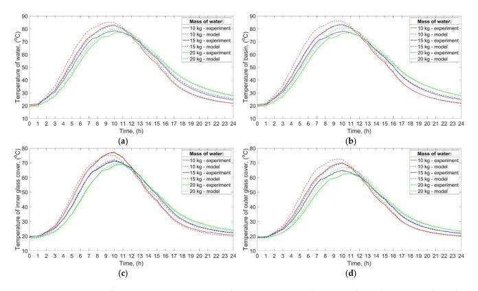
**Figure 9.** Temperatures of: (**a**) Water; (**b**) Basin; (**c**) Inner glass cover; (**d**) Outer glass cover; obtained experimentally and theoretically in the function of time for different water masses and high power of the electric heaters.
