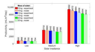
Figure 11. The comparison of SS's productivity for different water masses and different solar irradiances.
