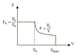
Figure 2. Traction performance curve.
