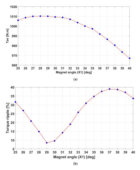
Figure 4. Impact of the side magnet angle variation on: (a) the average torque; (b) the torque ripple.
