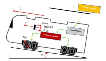
Figure 1. Electric traction system.
