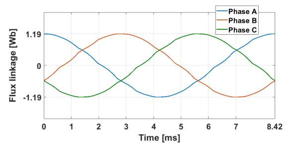
Figure 12. Stator winding flux linkage for the optimized structure.
