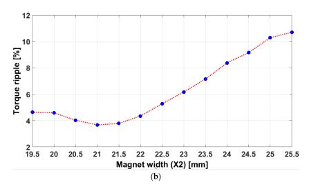
Figure 5. Impact of the side magnet width variation on: (a) the average torque; (b) the torque ripple.
