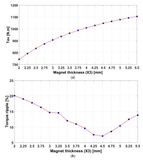
Figure 6. Impact of the side magnet thickness variation on: (a) the average torque; (b) the torque ripple.
