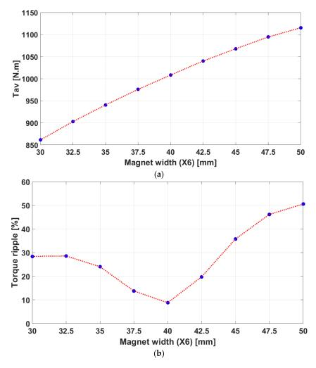
Figure 9. Impact of the central magnet width variation on: (a) the average torque; (b) the torque ripple.
