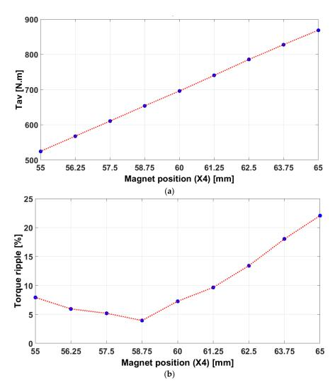
**Figure 7.** Impact of the central magnet position variation relative to the rotor center on: (a) the average torque; (b) the torque ripple.
