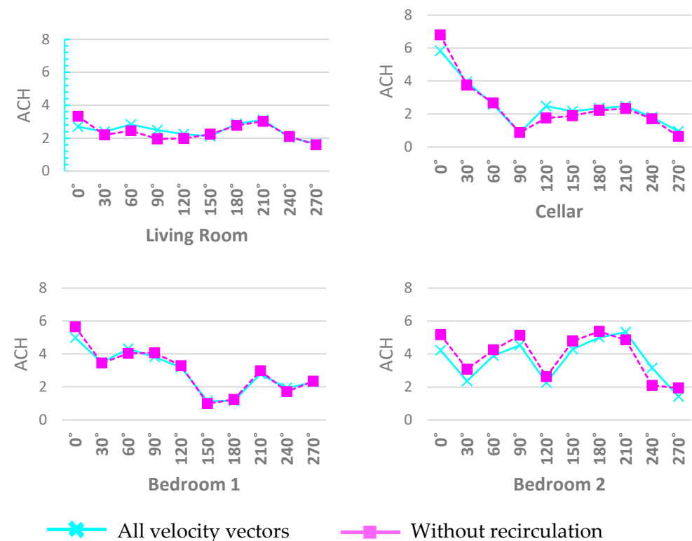
Figure 15. Predicted ACH at living room, cellar, and bedrooms 1 and 2—comparison between two approaches of the integration method.
