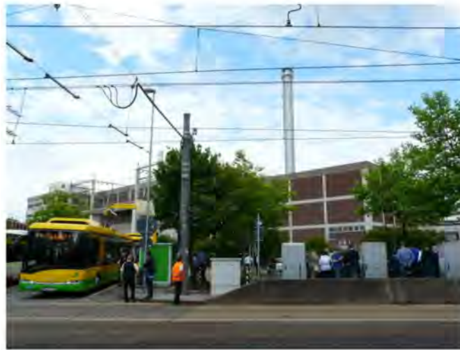
Figure 3. Charging station for electric bus and electric cars powered from the tram overhead line in Oberhausen, Germany.
