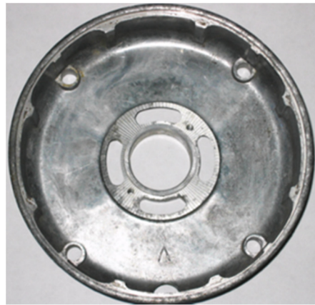
Figure 1. General view of the end shield of an electric motor, outer diameter 30 cm.
